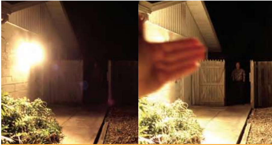
Glare from unshielded lighting reduces safety.
